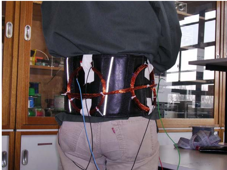
Figure 7.1 — Prototype of body-mounted magnetic tracking system with coils integrated in a belt.
