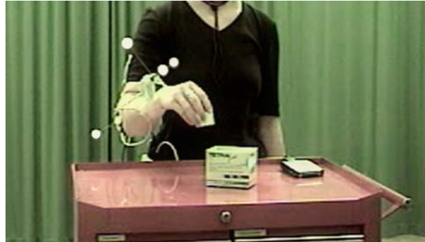
Figure 3.2 — Experimental set-up: the sensors module was placed on the wrist of the subject. Markers for the video-based reference system are indicated by the reflective dots. The object in front of the subject is an iron case that induced magnetic disturbances to the sensor measurements.
