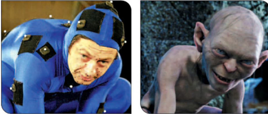
Figure 1.4 — Modern motion capture system used in film and game industries. Actor Andy Serkis in full motion capture suit, and right the CG mask of Gollum (Lord of the Rings).
